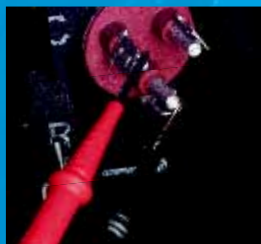
Ohm Out a Compressor
