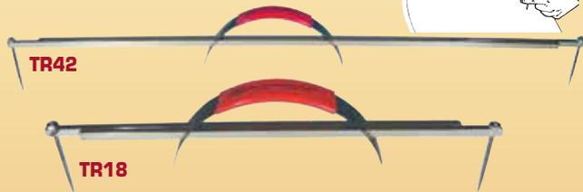
Two sizes handle a variety of layout applications. The TR42 expands to a big 42" (107 cm) radius (84" diameter). The compact TR18 expands to 18" (46 cm) and stores in most tool boxes. All steel construction. Points are resharpenable and also replaceable. Telescoping arms are nickel plated to resist corrosion. Handle features a comfortable vinyl grip.
