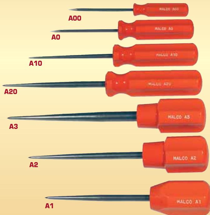
Use to scribe lines on metal, plastic and a variety of other materials. Pierce holes in wood, plastic, leather, - even light gauge metal. Blades are high carbon, alloy tool steel fully polished to resist rust. Blade tapers to a fine point and may be resharpened many times. Easy-to-spot orange handles are shock and shatter resistant. Shallow fluted handles with large end bearing surface provide a sure, comfortable grip. User has choice of large diameter or regular grip handles.
