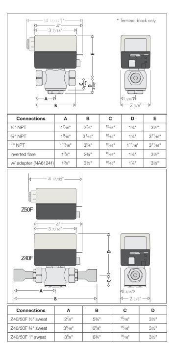
\*Inverted flare bodies ( 7/8" UNS female threads) with 2 attached copper sweat tailpieces:  $\ensuremath{\mathscr{V}}\xspace^*=$  Z20004X + (2) NA10005 field assembled
