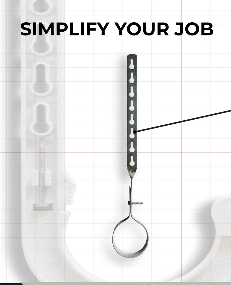
Our Patented Keyhole design allows for faster and easier installation which makes for a labor saving, more profitable job. Simply, pre-screw or nail the floor joists where the length of the pipe is to be installed, slip the hanger over the pipe and do not open the hanger. Lift the pipe by the hanger and slide the hanger over the screws that are mounted to the floor joists.
