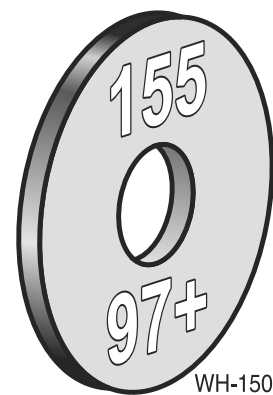
Figure 11 Propane gas orifice identification WM97+155
