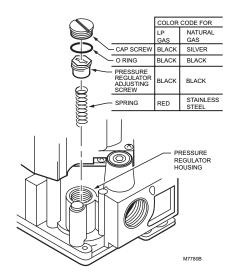
Fig. 2. Conversion kit installation in regulator.
