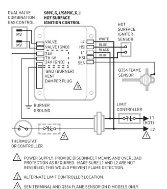
Fig. 9. Wiring connections for 24 volt control in S89C Direct Ignition System.
