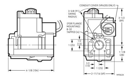
Fig. 1. Dimensions in in. [mm] of VR4205/VR8205 Combination Gas Control.
