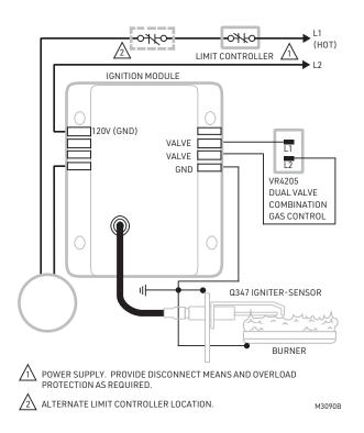
Fig. 7. Wiring connections for 120 volt control in direct ignition system.
