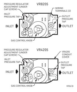
Fig. 5. Top view of gas control.
