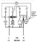
Wiring using 120V or 240V single phase line with
