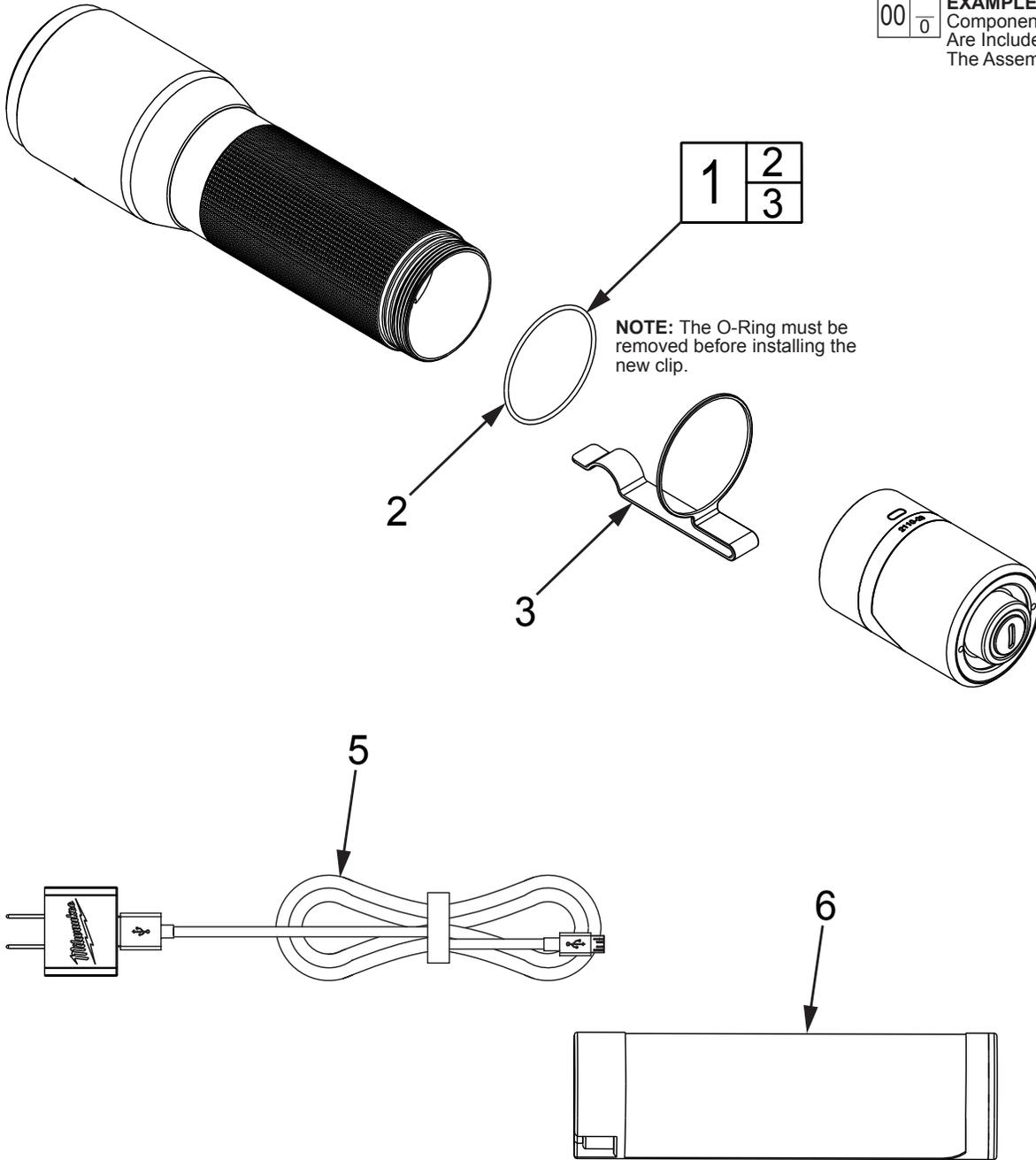
**NOTE:** The O-Ring must be removed before installing the new clip.
