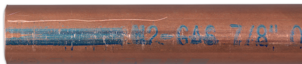
Figure 2 - Copper tube with "bad" surface scratch.
