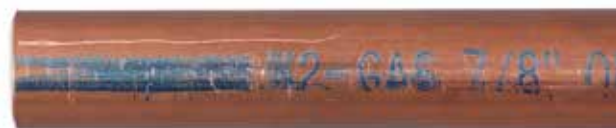
Figure 2 - Copper tube with "bad" surface scratch.
