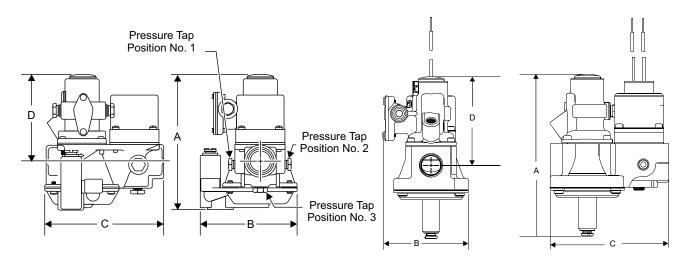
Bottom Adjust Regulator Model Showing Optional Pressure Tap Positions
