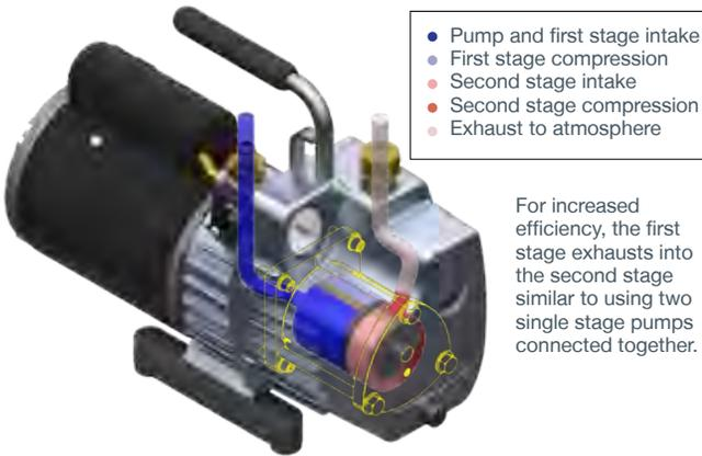
For increased efficiency, the first stage exhausts into the second stage similar to using two single stage pumps connected together.
