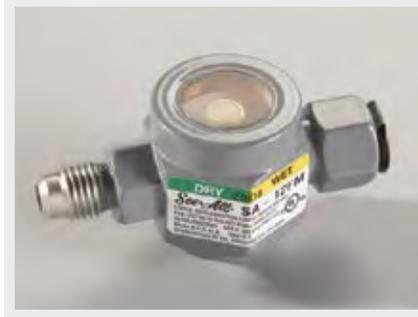
Use with YELLOW JACKET RecoverX and RecoverXLT machines. Indicates when all liquid has been recovered so you can switch immediately to vapor cycle and speed up the recovery process. 1/4" flare x 1/4" female flare.
