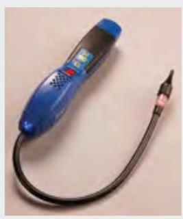
*The frequency of flashing from the electrolyte sensor tip increases as you get closer to a leak and refrigerant concentration increases. The audible alert, which can also be muted, increases in frequency and duration as concentration increases.*
