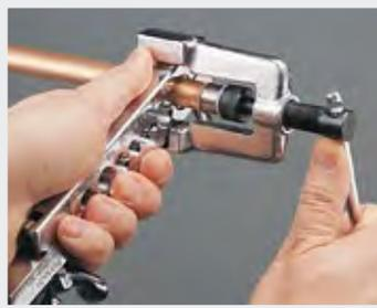
This combination tool both flares and swages soft or annealed copper and similar materials.
