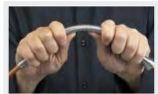
Spring benders slip over soft copper and aluminum tubing during bending to help prevent tube collapse.
