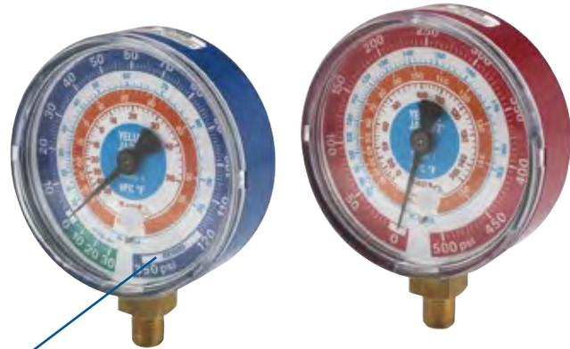
When a gauge has a **RETARD zone**, full scale is considered to be the last marked reading prior to entering the RETARD zone. For example, this gauge has a full scale reading of 120 psi. Gauge accuracy is not specified in the RETARD zone.
