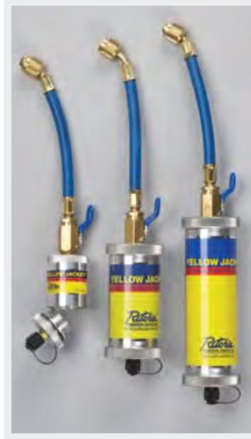
Body and cap are rugged aluminum with an "O" ring seal. 1/4" Male fitting at one end with Schrader. A ball valve for control on other end with a short length of hose. Valve depressor in 1/4" Female end. 600 psi working pressure.
