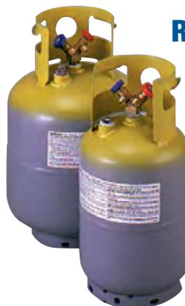
These gray and yellow 30 and 50 lb. cylinders feature "Y" valve for liquid/vapor, 400 psi rating and 3/4" plug for a float switch.
