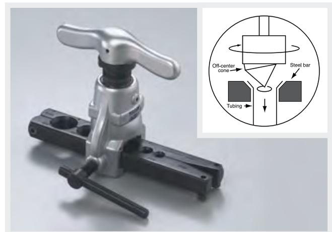
Off-center hardened steel cone with 45° flare produces a rolling action for uniform flare walls without galling in 3/16" to 3/4" O.D. tubing.
