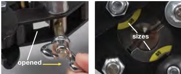
1. With cone up, open the two dies of the clamping yoke
