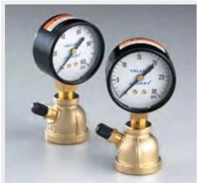
Easy-to-read gauge to test system pressure for leaks in new installations. Pressure drop indicates leakage. 0-30 gauge is in 1/4 lb. increments and 0-15 gauge is in 1/5 lb. increments. Brass threaded bell for leak tight connection.
