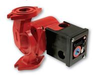
NRF-VS Pump Control is a versatile variable speed control for use in hydronic heating and cooling applications. Water temperature is controlled by regulating the speed of the pump which injects water from a different temperature water loop into a controlled loop.
