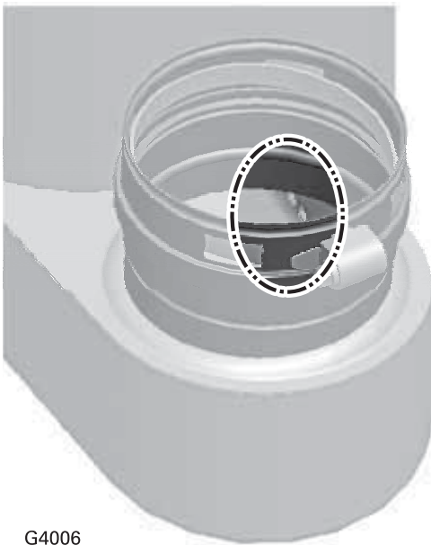
Figure 83 Recuperator flueway drain holes
