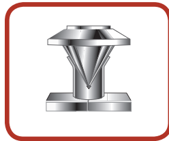
Flares rolled out above die bar.
