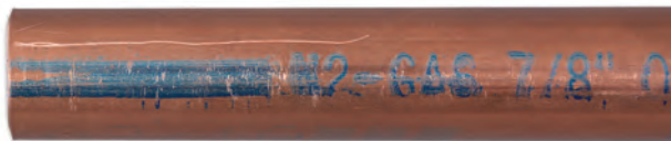
Figure 2 - Copper tube with "bad" surface scratch.
