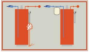
Adding a backflow preventer, check valve or water meter with a check valve creates a closed loop system. When water heats up, it expands with no place to go except through the relief valve. Installing a PH series thermal expansion tank on the cold water inlet provides a reservoir for water expansion. Water safely enters the tank and is released back into the system on demand.
