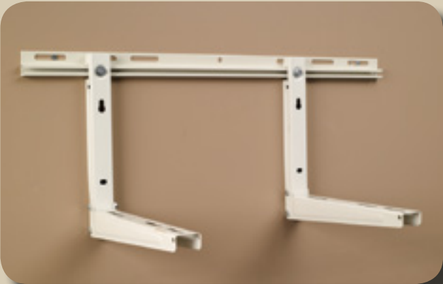
HEF-T-BRACKET™ TYPE 2 These brackets feature a cross bar that is attached to a wall and two L-shaped brackets that are hooked and bolted into place on the cross bar.
