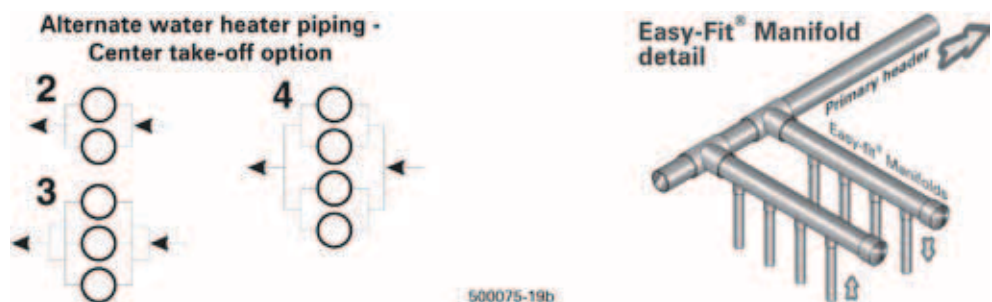
Figure 13 Alternate methods of revers-return piping and Easy-Fit® Manifold detail
