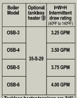
Tankless heater tappings are 3/4" NPT, with 3/4" NPT tapping for tankless temperature control.
