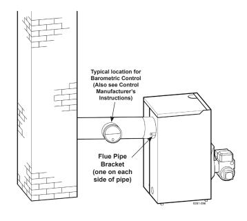
Figure 2b Top outlet breeching connection (only with optional "Top Vent Service Kit").
