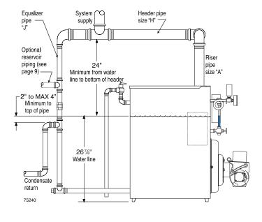
Figure 5 Recommended piping, OSB-3, -4 and -5, piping for parallel-flow systems only
