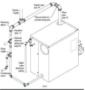
Figure 6 Recommended piping, OSB-6, piping for parallel-flow systems only
