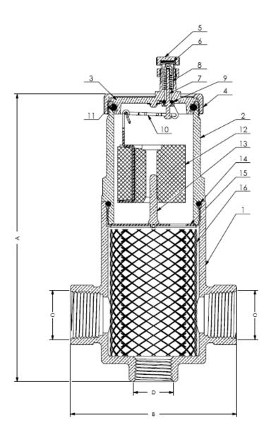
**Specifications:** Designed for residential, commercial or industrial use to quickly extract micro bubbles and static air from a hydronic heating system. The Air Separator must be installed in a straight run of horizontal piping and positioned precisely upright. Designated lengths of straight piping before and after the unit are not required. Neither side is designated as an inlet or outlet; the flow may be directed in either direction. Threaded ends comply with ANSI B1.20.1.
