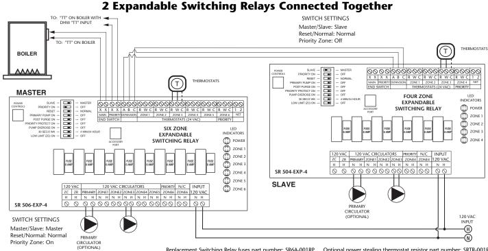
Replacement Switching Relay fuses part number: SR6A-001RP (Manufacture: Littlefuse, Part Number: 229006) Optional power stealing thermostat resistor part number: SRTR-001RP (Value: 1000 Ohms, 1/2 watt or higher)
