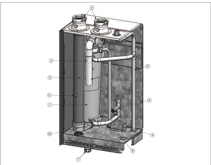
Fig. 7: PRESTIGE Solo 60 Internal Components
