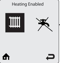
Domestic Hot Water Operation can be enabled and disabled by selecting the faucet icon and pressing the **OK** button to toggle operation between enabled and disabled. A faucet icon with an X through it indicates that the domestic hot water function is disabled. This icon is also displayed on the Home Screen when disabled.
