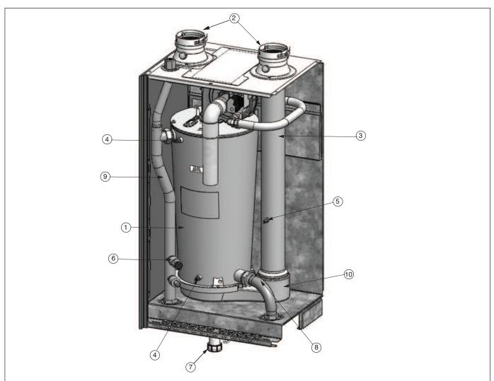
Fig. 9: PRESTIGE Solo 175/250 Internal Components
