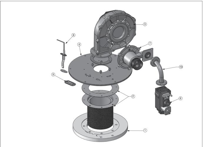
Fig. 14: PRESTIGE Solo 399 Burner Components
