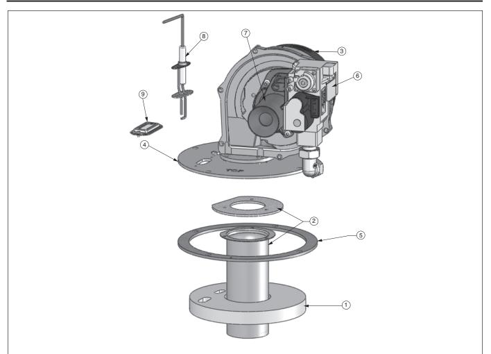
Fig. 13: PRESTIGE Solo 110 / Excellence Burner Components
