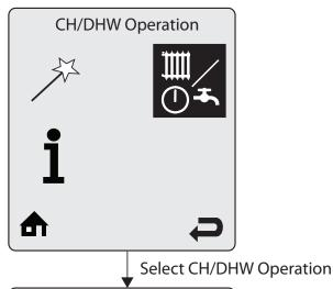
Heating Operation can be enabled and disabled by selecting the radiator icon and pressing the **OK** button to toggle operation between enabled and disabled. A radiator icon with an X through it indicates that the heating function is disabled. This icon is also displayed on the Home Screen when disabled.
