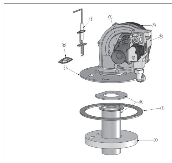
Fig. 12: PRESTIGE Solo 60/175/250 Burner Components
