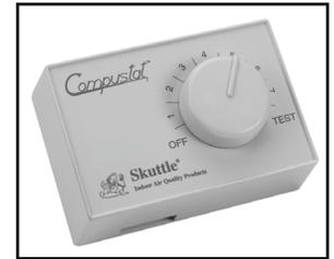
*Compustat* is an electronic compensating humidistat which automatically adjusts the humidifier output to compensate for changes in outdoor temperature. It helps prevent over-humidification in the event of a sudden outside temperature drop.
