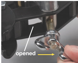
1. With cone up, open the two dies of the clamping yoke
