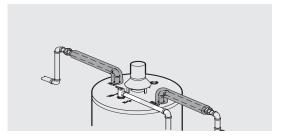
Typical horizontal piping arrangement
