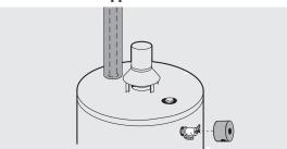
Typical Side Connect T & P Arrangement.
