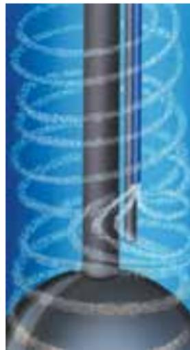
The spiraling effect also creates better mixing throughout the water heater tank which reduces the effects of stacking. Stacking occurs when frequent small draws of water create different temperatures throughout the tank resulting in increased peak temperatures at the top of the tank. The EverKleen™ system greatly reduces peak temperatures, thus increases first hour deliverability.
