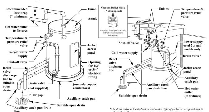
A new combination temperature and pressure relief valve, complying with the Standard for Relief Valves and Automatic Gas Shut-Off Devices for Hot Water Supply Systems, ANSI Z21.22, is supplied and must be installed in the opening provided and marked for the purpose on the water heater. No valve of any type should be installed between the relief valve and the tank. Local codes shall govern the installation of relief valves.
