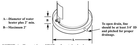
NOTICE: Auxiliary catch pan MUST conform to local codes. Catch Pan Kits are available from the store where the water heater was purchased, or any water heater distributor.
