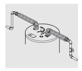
Typical horizontal piping arrangement
