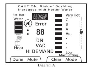
User Mode is entered after all required data is received from the appliance when powered-up. The display shows temperature setpoint, estimated amount of hot water and maximum temperature setpoint. Heat symbol is turned on when heating cycle is active. Scald warning starts flashing whenever the adjusted setpoint exceeds the "Hot" setting and becomes solid after 30 seconds of flashing.
