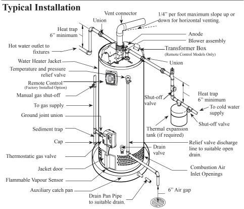
A new combination temperature and pressure relief valve, complying with the Standard for Relief Valves for Hot Water Supply Systems, ANSI Z21.22/CSA 4.4, is factory installed and must remain in the opening provided and marked for the purpose on the water heater. No valve of any type should be installed between the relief valve and the tank.
