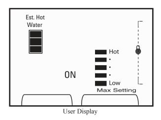
The water heater gas valve knob below is set to VERY HOT therefore the user display shows Very Hot as the maximum available setpoint. The customer in this example has chosen to set the temperature between
