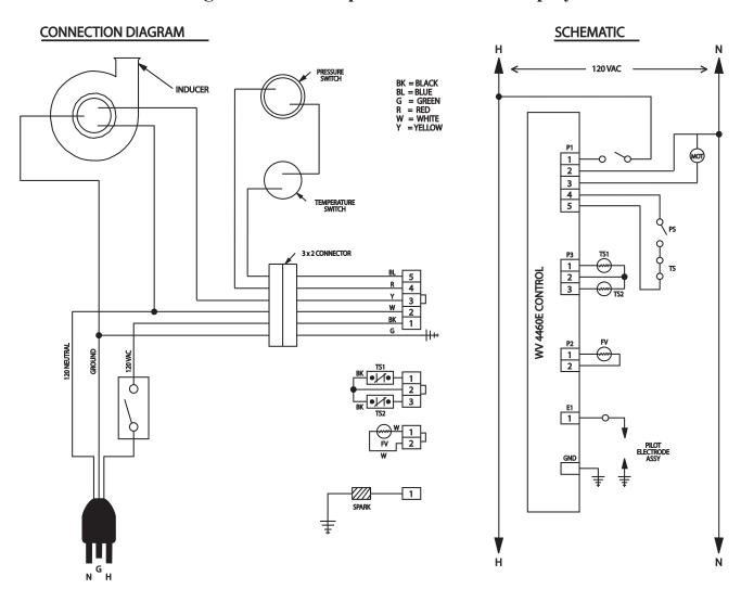
▲ CAUTION! Label all wires prior to disconnection when servicing controls. Wiring errors can cause improper and dangerous operation. VERIFY PROPER OPERATION AFTER SERVICING!
