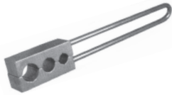
MLP3C CRIMPING TOOL To be used with 3/16", 1/4", and 3/8" ID hose ferrules. Strike with hammer or press in vise, then turn 90° and strike or press again.
