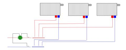
Pensotti recommends their panel radiators be connected to the piping system through the bottom supply and return connections. This guarantees complete water flow through the radiator and proper operation of the flow-setter and thermostatic valve.
