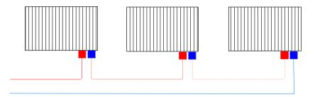
Series Circuit w/ By-Pass Valves (Maximum Circuit Flow Rate Is 2 GPM, And / Or 4 Radiators)
