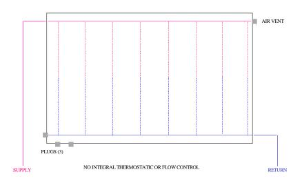
PENSOTTI PANEL RADIATORS - ALTERNATE PIPING ARRANGMENT 1
