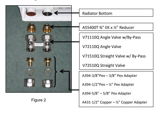
**Figure 1 Pex**: Insert the A55400T reducers into the supply and return connections of the radiator and tighten with a 12mm allen wrench. Choose the proper size pex tubing adapter assembly, slide the nut
