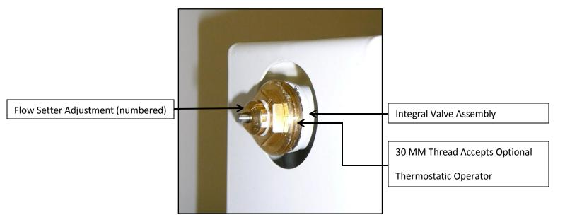
Flow Setter is adjusted by turning the inner gland (picture above) to the corresponding number.
