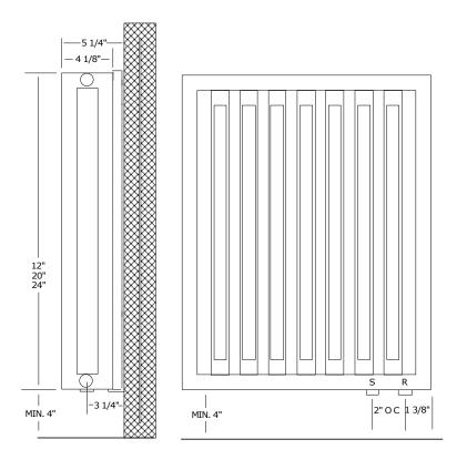
Radiators should be placed on an outside wall, below a window if possible. Check the installation location and determine if adequate space is available to accommodate the panel size chosen.
