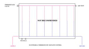
PENSOTTI PANEL RADIATORS - ALTERNATE PIPING ARRANGEMENT 4
