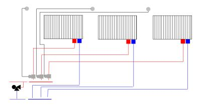
Homerun with Thermostatic Operators and Variable Speed Delta T Circulator
