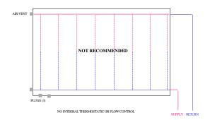
PENSOTTI PANEL RADIATORS - ALTERNATE PIPING ARRANGEMENT 4
