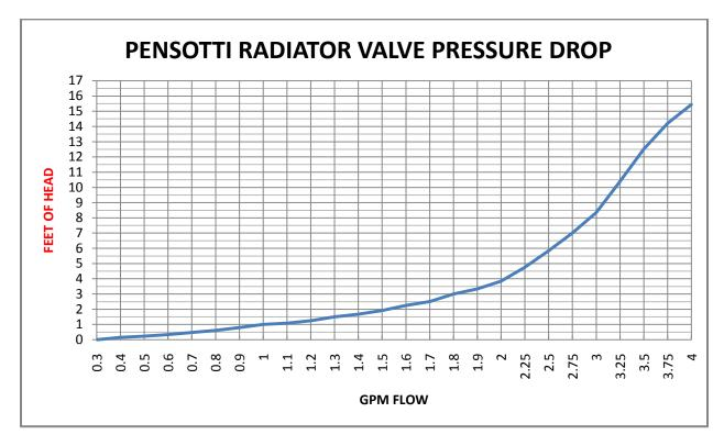
Determining the pressure drop for the radiator valve is the same procedure used for the radiators on the previous page. Find the calculated flow rate in Gpm on the bottom axis of the chart, move straight up until you intersect the curve then draw a line to the left axis and read the pressure drop in feet of head.
