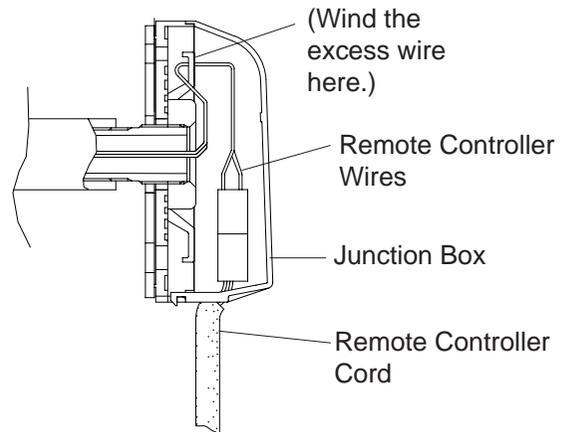
3. Insert the wall pipe containing the remote controller wires through the hole.
