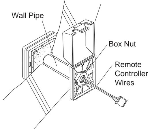
2. Drill a  $\varnothing 1\text{-}1/4\text{'}$  hole in the wall where the remote controller will be installed.
