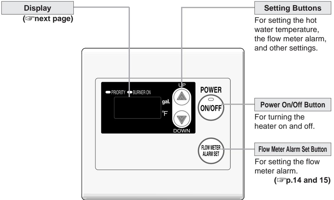
\* Before use, remove the protective sheet from the remote controller surface.
