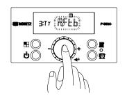
7. With '3:TY' displayed, press the 'Dial Button'. 'A:Ftb' will begin flashing (default). Turn the 'Dial Button' clockwise to select the appropriate heating system type. Press the 'Dial Button' to confirm the setting.
