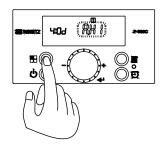
19. To return to the 'Installer Mode' main menu, press the 'Function Button'. Use the 'Dial Button' to scroll through the other menu options. To exit 'Installer Mode', press the 'Function Button' once more.
