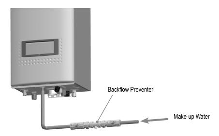
• External water feeder may be installed on the system piping if it is required for specific applications. See the following figure for an example of external water feeder installation on the system piping.
