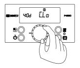
16. Turn the 'Dial Button' until 'C.Lo' is displayed. 'C.Lo' allows for adjustment of the design low temperature setting.
