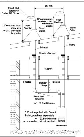
When choosing intake and exhaust terminations, you must use the same type of elbow (i.e. both 90° elbows). This will help with proper combustion by putting both terminations in the same pressure zone.
