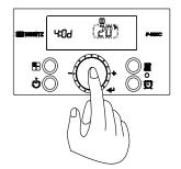
17. Press the 'Dial Button'. The default design cold weather temperature (20°F) will flash on the display. Turn the 'Dial Button' to adjust to the desired temperature.
