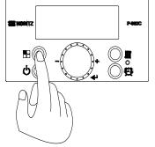
1. Turn off the power to the control panel. Press and hold the 'Function Button' for approximately 5 seconds to get into the 'Installer Mode'.
