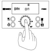
4. Press the 'Dial Button' to save the setting. If you would like to move to next function in the 'Installer Mode', turn the 'Dial Button' clockwise or to exit 'Installer Mode' press the 'Function Button'.
