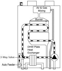
2) When the water filling is finished, then the 3-Way Valve will be switched to heating supply pipe and proceed to add water to increase the pressure on the heating loop.
