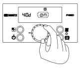
14. Press the 'Dial Button'. The default setting of ON will begin to flash on the display. Turn the 'Dial Button' to OFF if desired.
