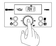
9. With '4:Od' displayed, press the 'Dial Button'. 'A:HI' will begin flashing.
