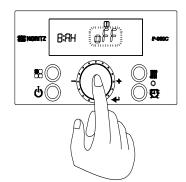
3. Press the 'Dial Button' so 'oFF' is blinking. Then turn the 'Dial Button' clockwise so 'on' is blinking.
