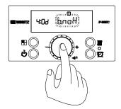
13. Press the 'Dial Button'. 'b:noH' will being to flash on the display.
