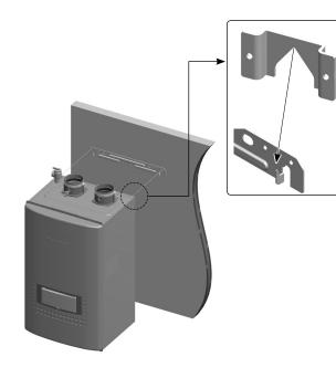
9. Place the Combi Boiler back on the wall. (same as step 5)10. Screw in the two screws into the dry wall anchors.
