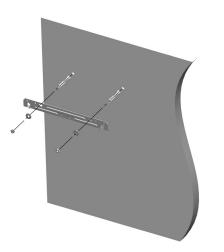
6. Locate the lower mounting bracket on the bottom of the Combi Boiler. The two screws and dry wall anchors will be used to securer the bottom of the unit to the wall.
