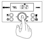
'0-2' will flash when the 'Dial Button' is pressed. (The default setting is '0-2' for installations at 0~1,999ft elevation.)
