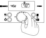
10. Press the 'Dial Button'. The default design warm weather temperature (70°F) will flash on the display. Turn the 'Dial Button' to adjust to the desired temperature.
