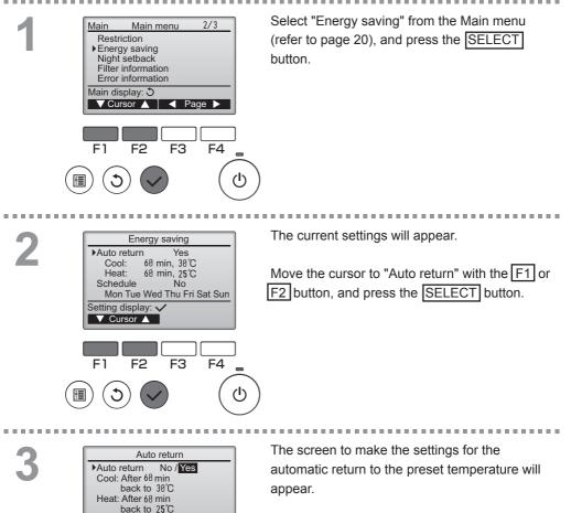
Move the cursor to the desired item with the F1 or F2 button out of "Auto return," "Cool," or "Heat."
