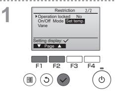
To enable the operation lock function, set the item "Operation locked" to " Yes".
