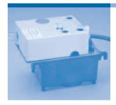
The SRP-1 is a small, sealed reservoir pump designed to collect and pump melt/flush waste from small under counter cube machines (Whirlpool, Scotsman, GE, Hotpoint). The pump is small enough to fit most installations, and the unique sealed reservoir prevents overflow despite the low tank capacity. Available in 115V only. Part No. 801074
