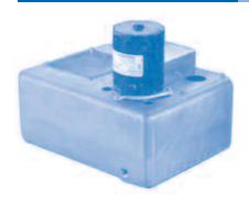
Hartell's AL-2 series pumps are designed to handle the high volume of water produced during the flushing cycle. The AL-2 comes with a 2 gallon cast aluminum reservoir, 6 foot cord and plug, 1 3/8" inlet and 3/8" NPT Female outlet. Maximum water temperature 150° F.
