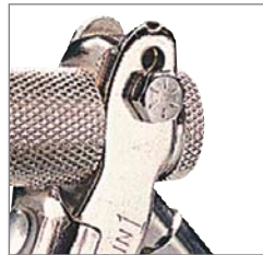
SHORT "RATCHET ACTION" POWER STROKE Bolt in lower hole for hard pulling rivets in several easy pulls.
