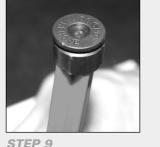
To separate the SWITCH ASSEMBLY (21) prior to installation, place the SWITCH ASSEMBLY (21) on the LONG PIN TOOL.
