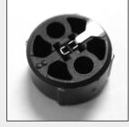
**STEP 11** The LOWER INSULATOR (15) should look like this. Note that the SIDE CONTACT (13) comes to the rim of the insulator.
