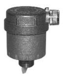
MODEL T-70 **LEGEND MODEL T-70** automatic hot water air vent is constructed of heavy duty forged brass. It features a low profile, compact body with side vent designed to fit anywhere. It removes air from tanks, baseboards, radiators, unit heaters and systems. It is used for continuous venting of hot water and chilled water systems.
