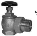
MODEL T-431 **LEGEND MODEL T-431** steam angle radiator valves are constructed of heavy duty bronze. They have a screwed bonnet, rising stem and composition disc. **LEGEND MODEL T-431YB** (Yellow Brass) is the same heavy pattern as the T-431 except it is brass instead of bronze. Each valve is tested twice: air under water, in the open and closed position .
