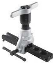
T30600 Ratcheting, eccentric cone flaring tool with internal clutch to prevent over-torquing. For tube OD: 3/16", 1/4", 5/16", 3/8", 1/2", 5/8" and 3/4"
