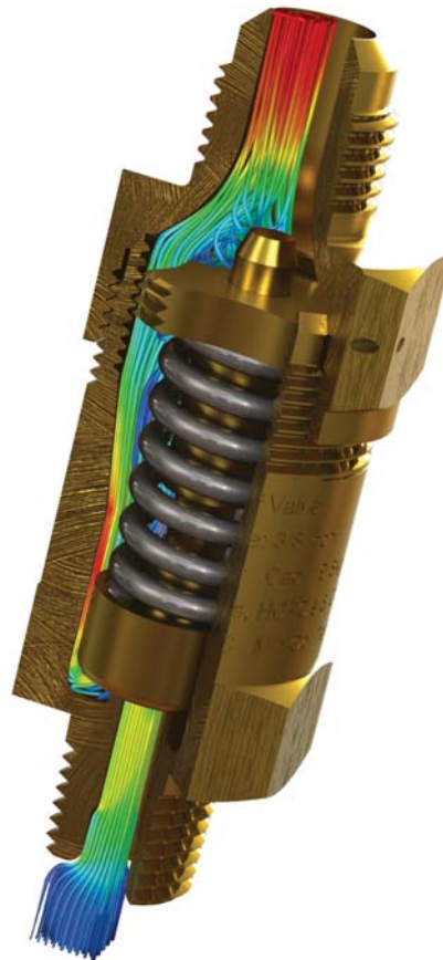
CFD - PRESSURE RELIEF VALVE
