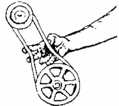
Too much deflection indicates the belt is not tight enough, which will result in slippage causing a loss of blower speed and belt failure.
