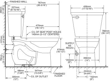
THIS TOILET IS DESIGNED TO ROUGH-IN AT A MINIMUM DIMENSION OF 305MM (12") FROM FINISHED WALL TO C/L OF OUTLET.
