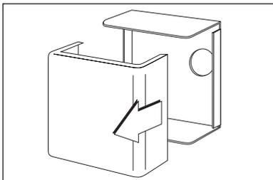
Loosen the two control box cover binding head screws and remove the cover.
