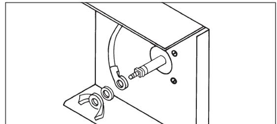
Connect the ring terminal wire lead to the probe terminal stud and secure with the lock washer and wing nut provided. *With the power removed*, proceed with installation and wiring according to Method A or B described on next page.
