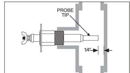
Check to insure 1/4" clearance from probe to any surface within the boiler or tee. When installed in a tee, the probe tip should extend fully into the pipe run. Apply pipe sealing compound to threads.
