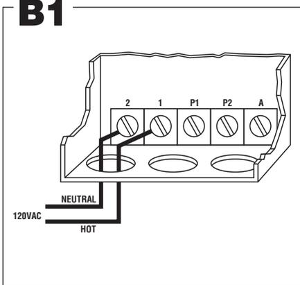
**◀B1** Connect the hot lead of the input voltage (120 VAC, 60 HZ) to terminal 1. Connect the neutral lead to terminal 2. 120 VAC, 60 HZ must be supplied to terminals 1 and 2 for internal operation of the control.
