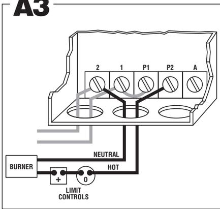
**◀A3** Connect terminal 2 to burner circuit neutral. Connect terminal P2 to burner circuit in series with other limit controls. Consult boiler manufacturer instructions for proper terminal connections. Control should be wired in series with and before other circuits.
