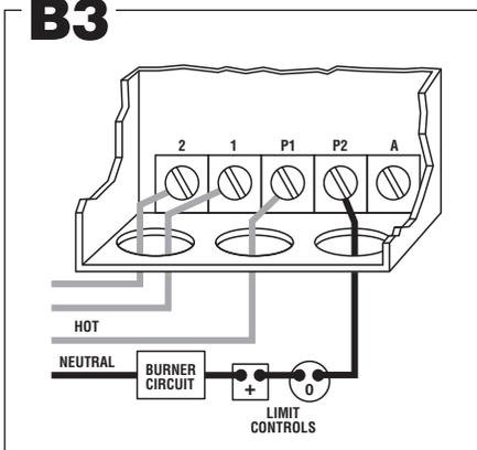
**◀B3** Connect terminal P2 to burner circuit in series with and before other limit controls.
