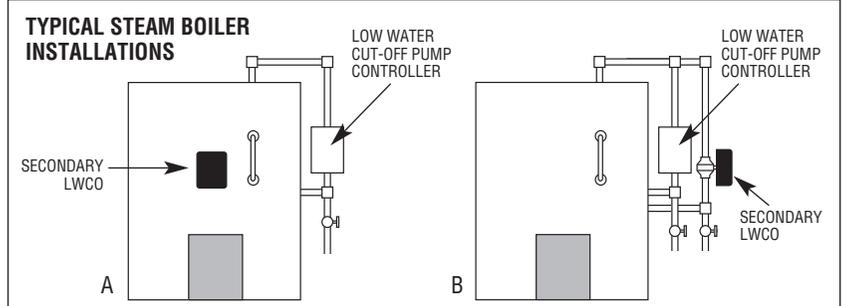
**STEAM BOILERS (Secondary):** Control must be installed in a suitable tapping provided in the boiler (A), or in an equalizing line (B). The control should be located below the level of the primary low water cut-off but above the lowest permissible water line as specified by the boiler manufacturer.
