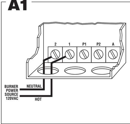
**◀A1** Connect the hot lead of the input voltage (120 VAC, 60 HZ) to terminal 1. Connect the neutral lead to terminal 2. 120 VAC, 60 HZ must be supplied to terminals 1 and 2 for internal operation of the control.
