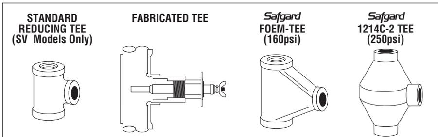
**TEE MOUNTING:** If a field fabricated tee is used, make sure that the tee drains thoroughly when the water level falls below it, and that it conforms to the spacing requirements described in Step 3. Models equipped with the shorter EL1214-SV probe can be installed in most standard reducing tees. Safgard cast iron tees are also available to accommodate all probe models (See page 4).
