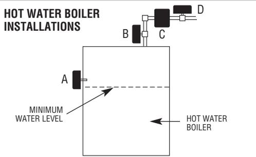
**HOT WATER BOILERS:** Probe must be installed at or above the minimum safe water level established by the boiler manufacturer. The probe may be installed directly in the boiler (A) if a suitable tapping is available, in the riser (B), in the header horizontally (C), or in the header vertically (D). **IMPORTANT:** To assure proper drainage, pipe diameter should be no less than 1" on installations in vertical piping and no less than 1¼" on installations in horizontal piping.
