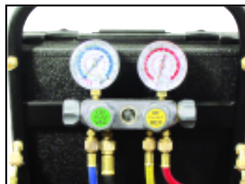
Hard mounted manifolds
