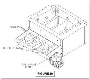
A visual check of the main burner and pilot flames should be made at the start of the heating season and again in mid-season. The main burner flame should have a well defined inner blue mantel with a lighter blue outer mantel. Check the burner throats and burner orifices for lint or dust obstruction. See figures 19 and 20 above.
