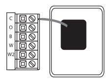
Insert 2 AA Alkaline batteries (included). High quality alkaline batteries are recommended.
