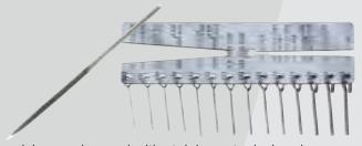
Precision engineered with stainless steel wire plugs. Features a specially designed file to cut and open tubes. The numbers are etched in black for better legibility. Fourteen ID sizes from 0.026 units to 0.090 units and 22 OD sizes from 0.072" to 7/16" (5 to 12 mm). Use both the ID and OD calibrations to correctly determine tube size. Place tube in "V" slot to measure OD. Pin gauge measures ID.
