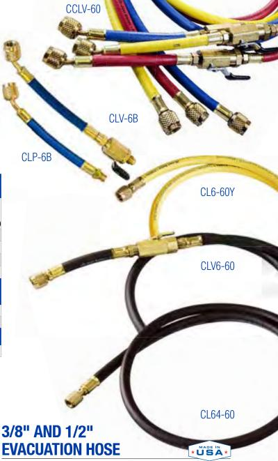
New heavy-duty evacuation hose features no valve core depressors for faster evacuation and deeper vacuums. The fittings are different on each end and handle 800 psi working, 4000 psi burst. Available in black only. Straight fittings by straight fittings.
