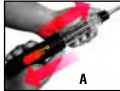
Pull handle back to return bit to storage chamber
